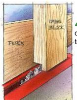
**4** Once again, the gauge block helps you precisely set up for a cut. Position it as shown left to reset the height of the dado set to 1/4" high. Do not change the position of the fence.
